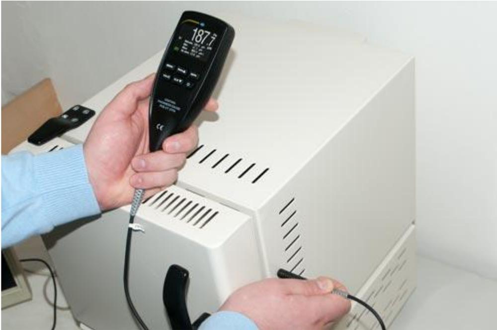
Here you can see the coating thickness gauge PCE-CT 27FN by checking of the paint thickness.
