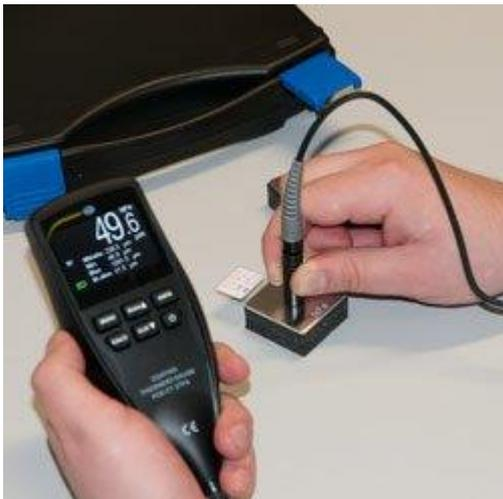
Here you can see the calibration of the coating thickness gauge
